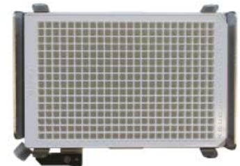
7000166 Footprint of CPAC with positioning frame
