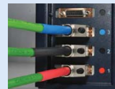
8900030 Multi TEC Control (MTC) with inserted slot modules and connected devices with corresponding color.
