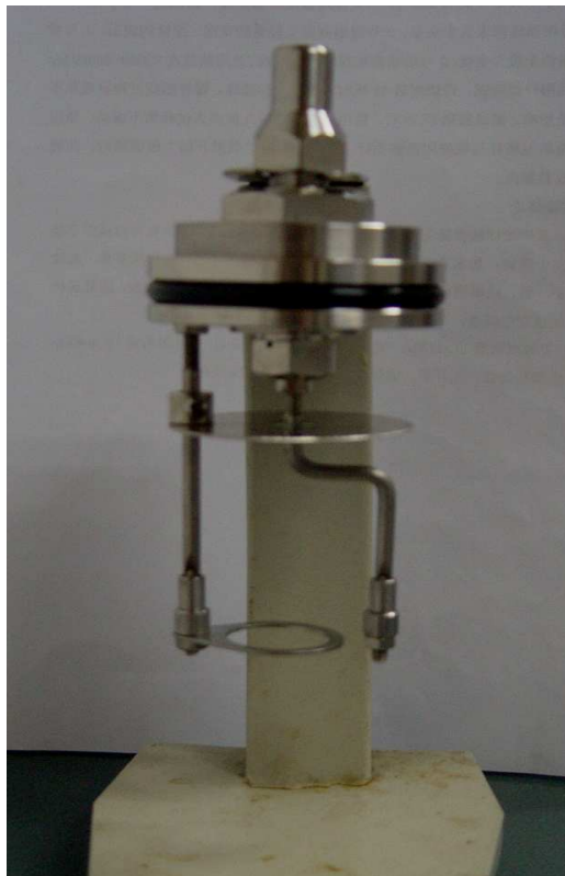
Fig. 2-4 Internal structure of Oxygen bomb
