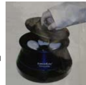
Rotor lid should be tied down
