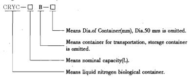
For example: CRYC-30 means the liquid nitrogen biological container with a nominal volume of 30L and a caliber of 50-mm, CRYC-50B-80 means the liquid nitrogen biological transporting container with a nominal of 50-L and a caliber of 80-mm.
