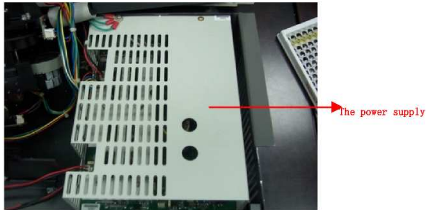
Figure 13.6 The power supply
