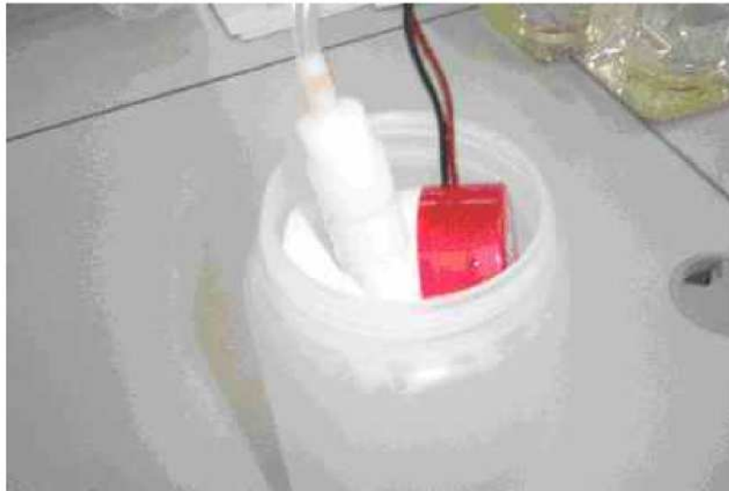
Figure 2.2 Place the pump into the wash bottle
